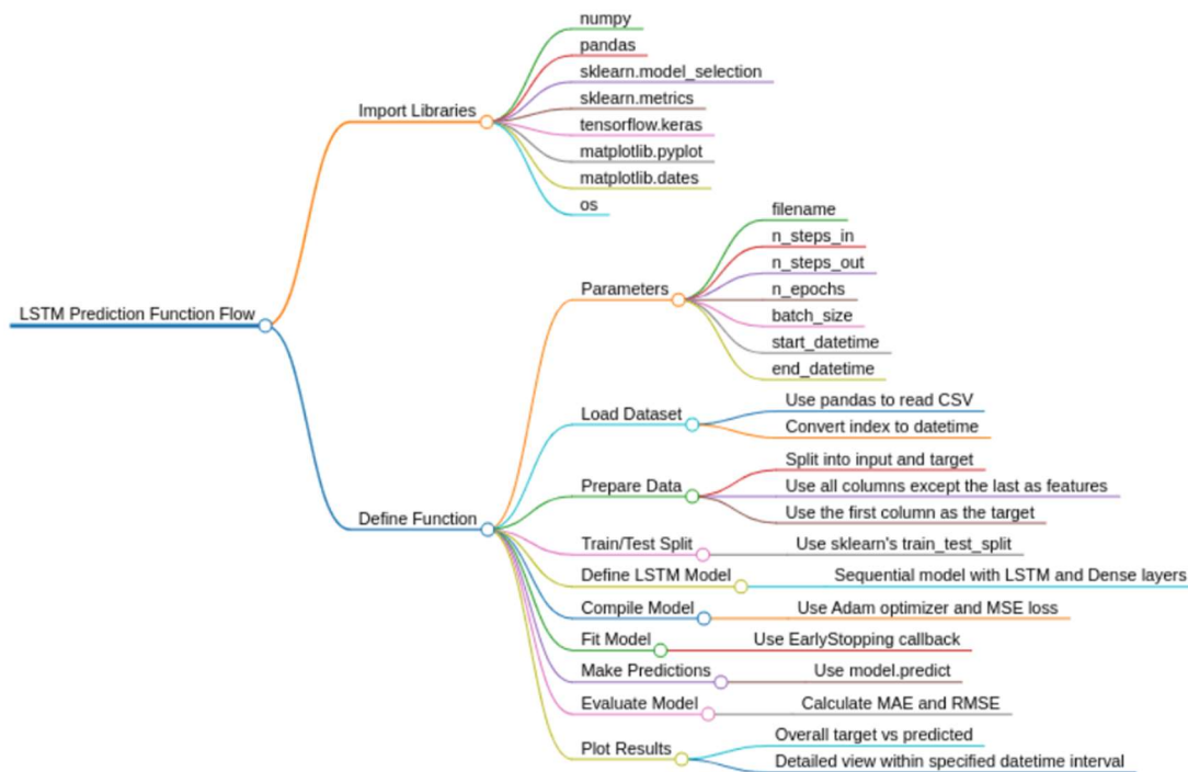
Figure 52. LSTM prediction process function diagram.
