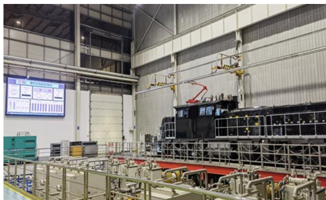
Locomotive #2 undergoing 25kV traction testing in Zhuzhou, China
