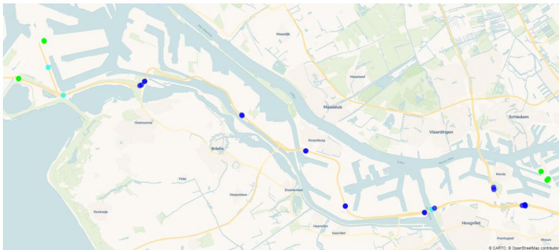
Figure 1 – Location of the sensors providing the measurement data. Blue sensors record aggregated vehicle counts, cyan sensors provide counts disaggregated into three vehicle classes, and green sensors differentiate up to five classes.
